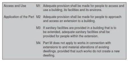
Figure 1 – The requirements of Part M (2010) of the Building Regulations
